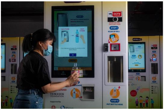
Press OK <u>after</u> you have collected and pasted the sticker(s) on the bottle(s), <u>within 45 seconds</u>. (Note: The machine will restart if you do not click OK after 45 seconds. If this happens, start again from Step 1.)
